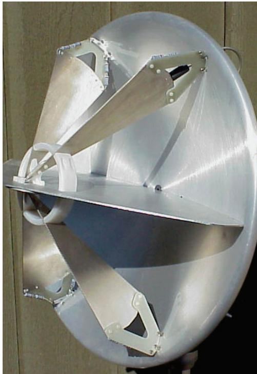
This recent design includes a ground plane that lies in a plane of symmetry, and does not affect the antenna.
