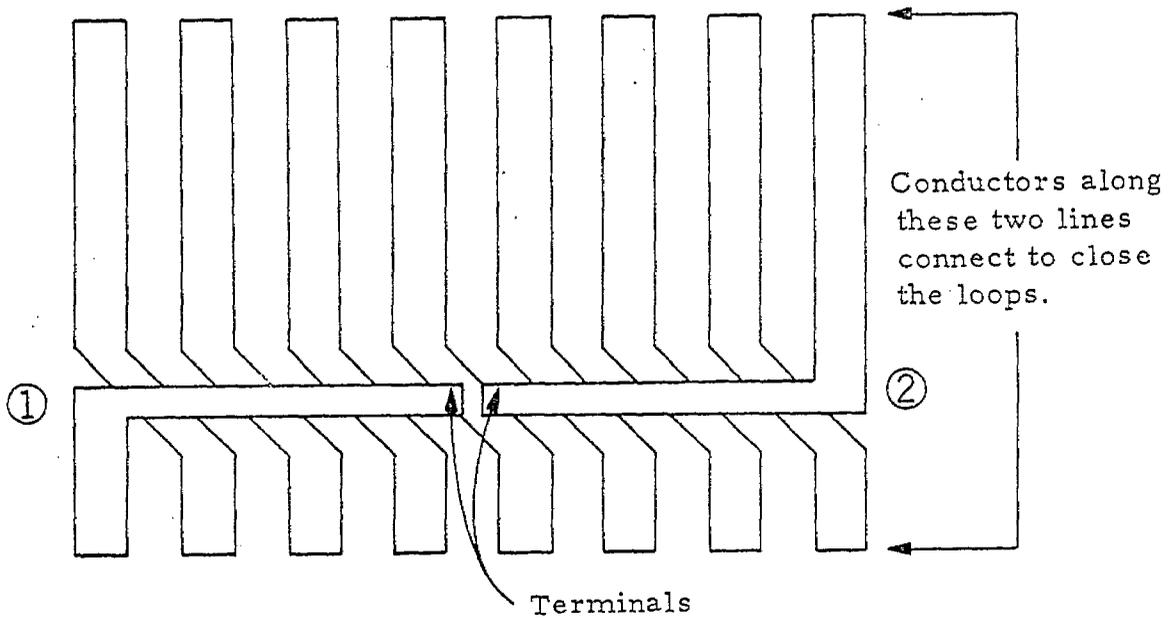
B. Terminals at ends of single winding:  $N=8$ : Expanded View
