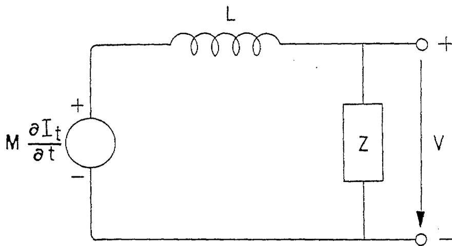
Figure 2. Equivalent Circuit for Inductive Current Sensor
