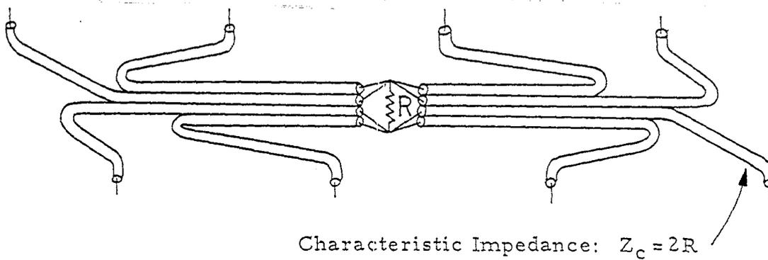
C. Signal cables laid out with termination
