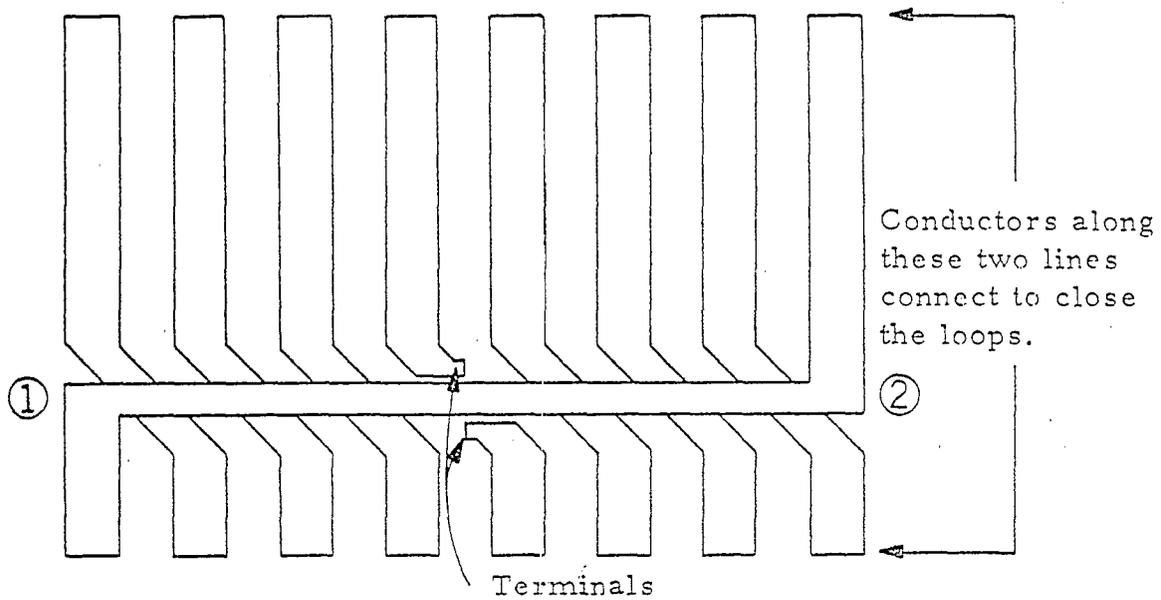
A. Terminals in center of single winding:  $N = 8$ : Expanded View
