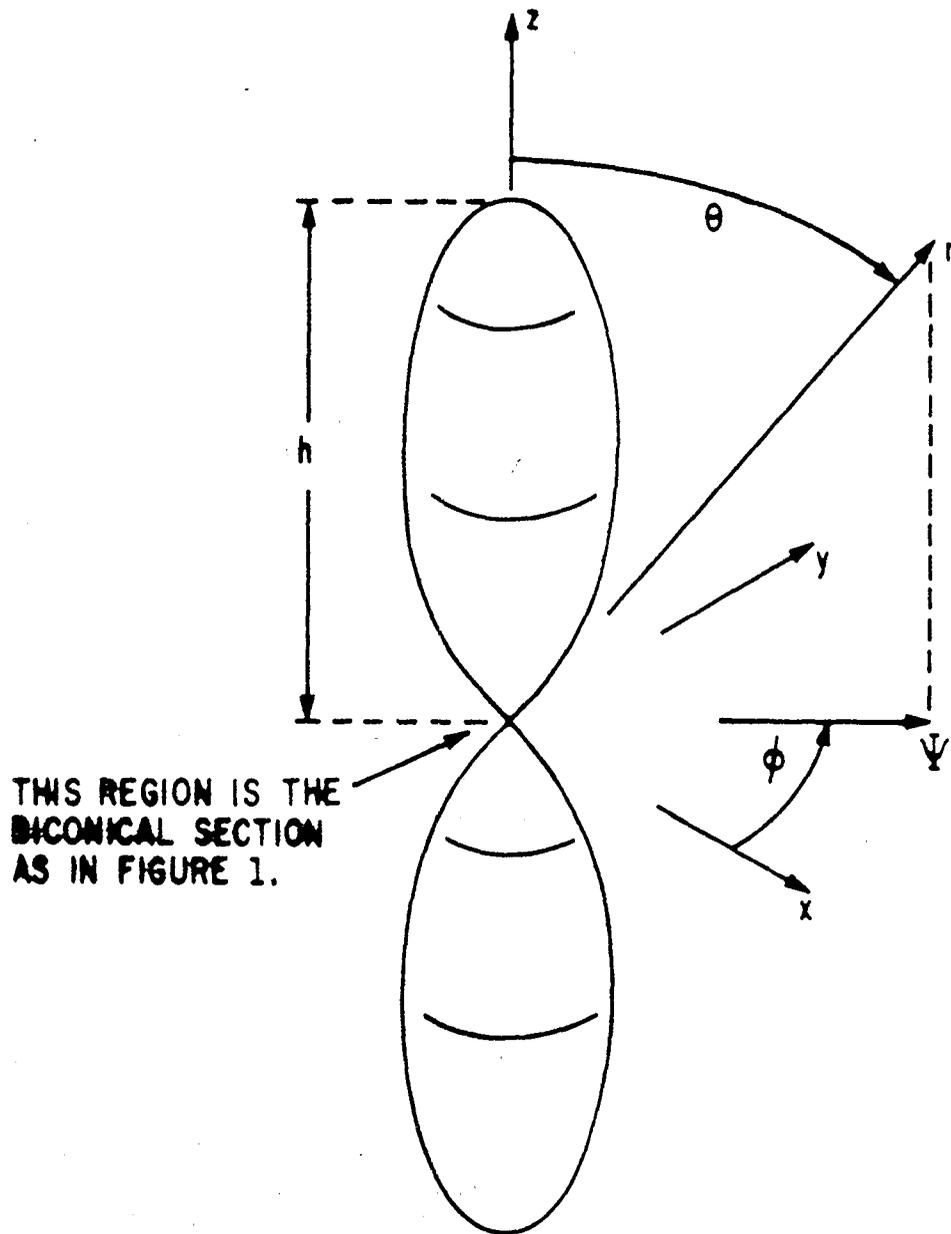
**FIGURE 2. AXIALLY AND LENGTHWISE SYMMETRIC PULSED DIPOLE ANTENNA**
