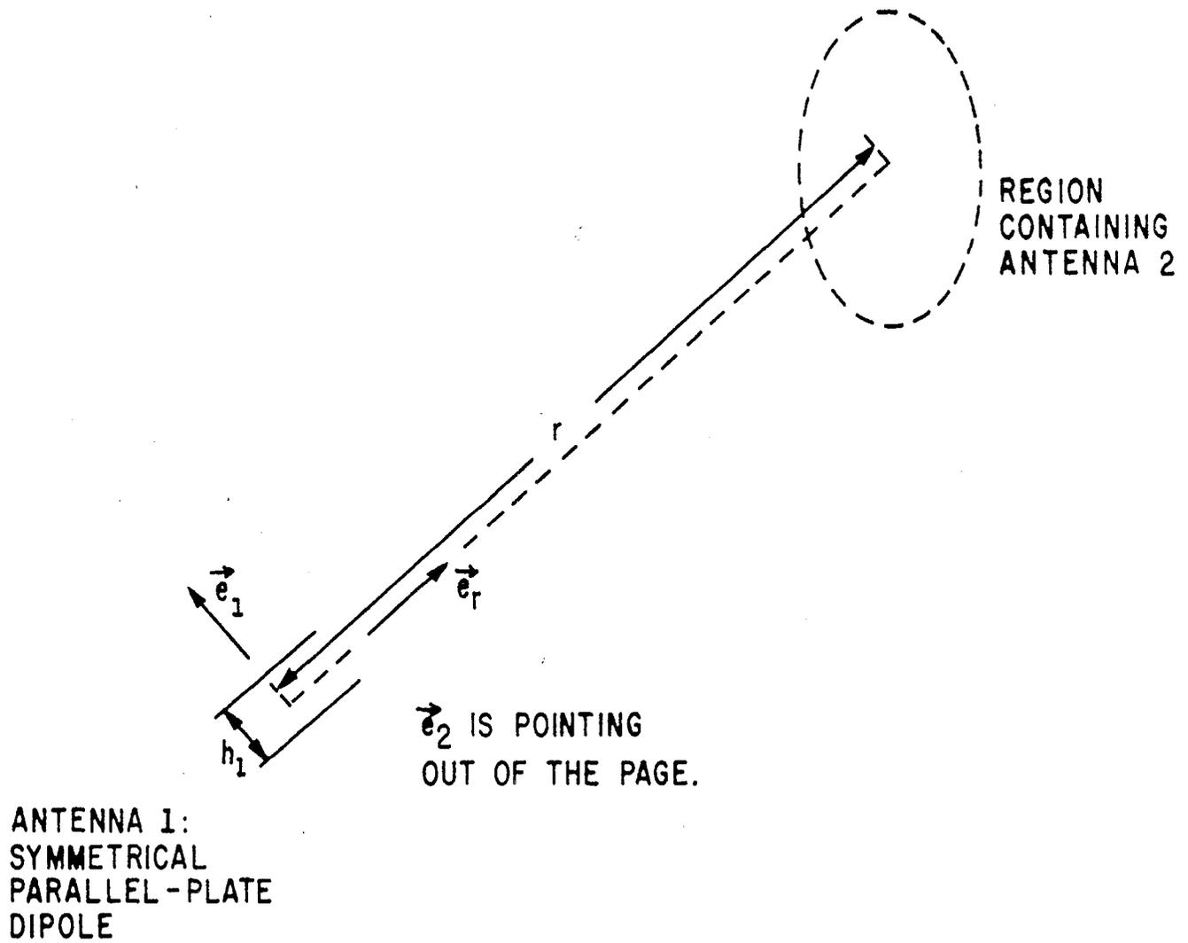
FIGURE 3. TWO DIPOLE ANTENNAS WITH COORDINATES
