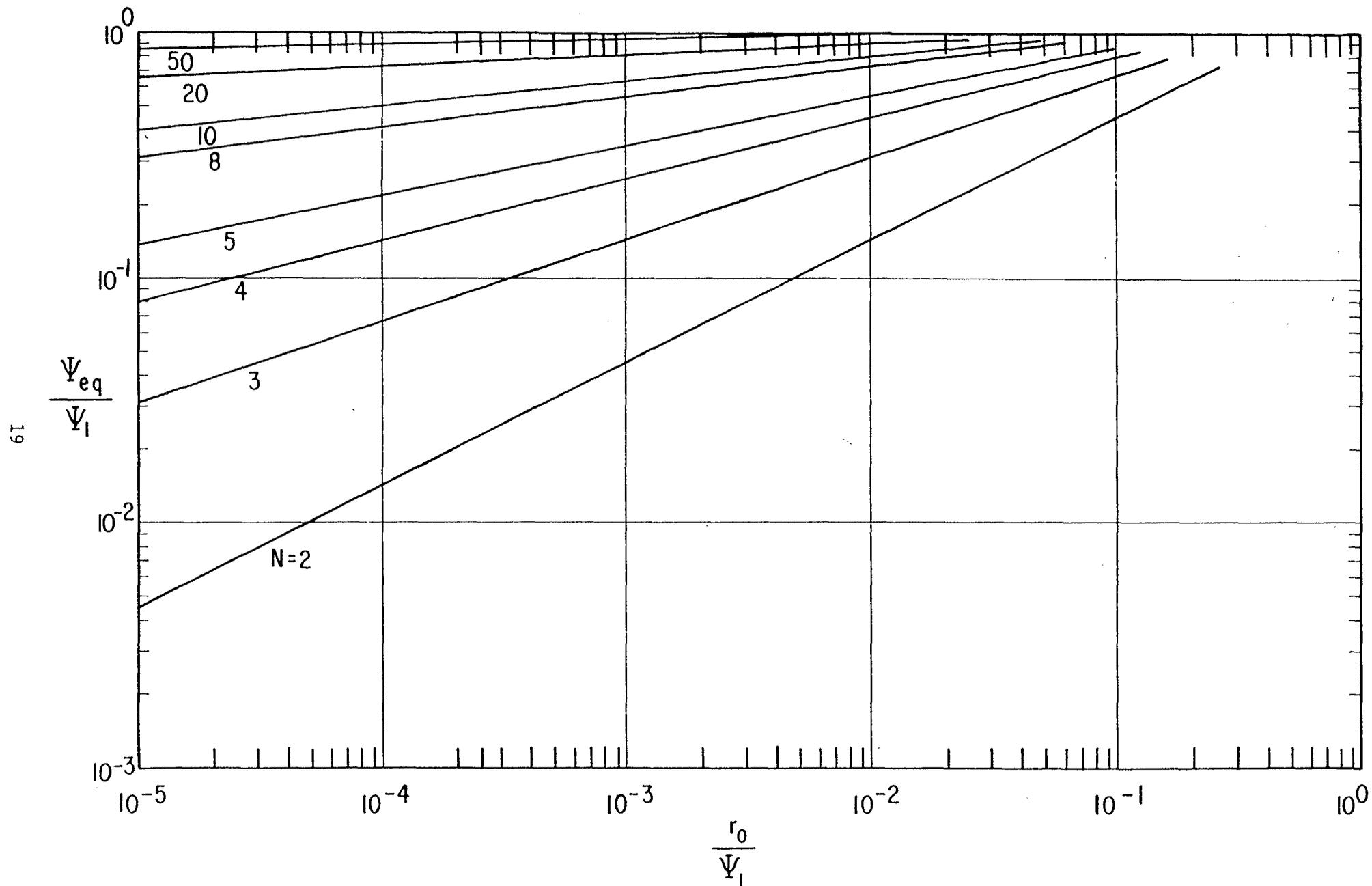
FIGURE 5. EQUIVALENT RADIUS OF WIRE ARRAY FOR VARIOUS  $N$
