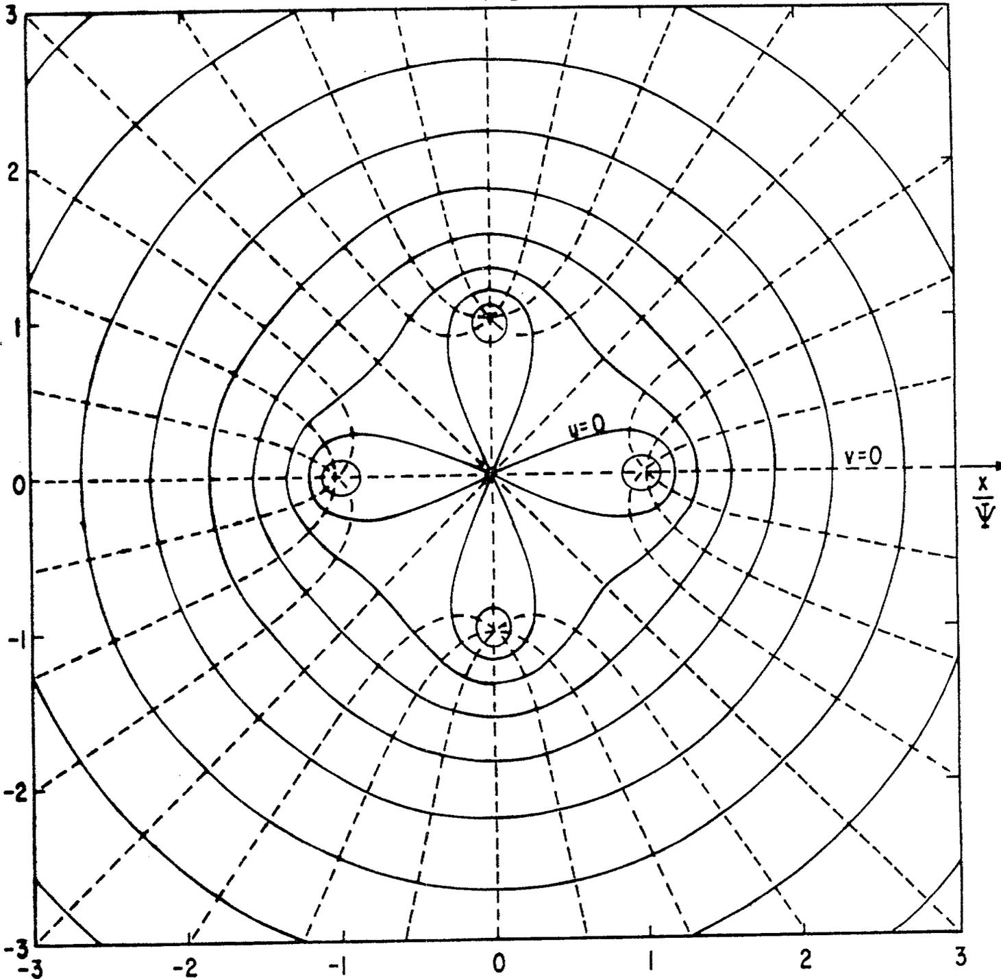
FIGURE 4. POTENTIAL PLOT FOR THE CASE OF FOUR WIRES
