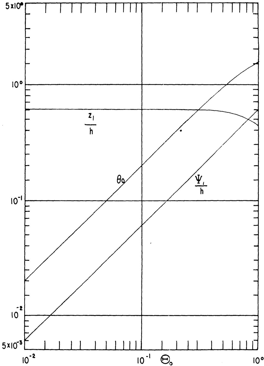
FIGURE 3. CONE ANGLE, MAXIMUM ANTENNA RADIUS, AND POSITION OF MAXIMUM AS FUNCTIONS OF  $\Theta_0$ .
