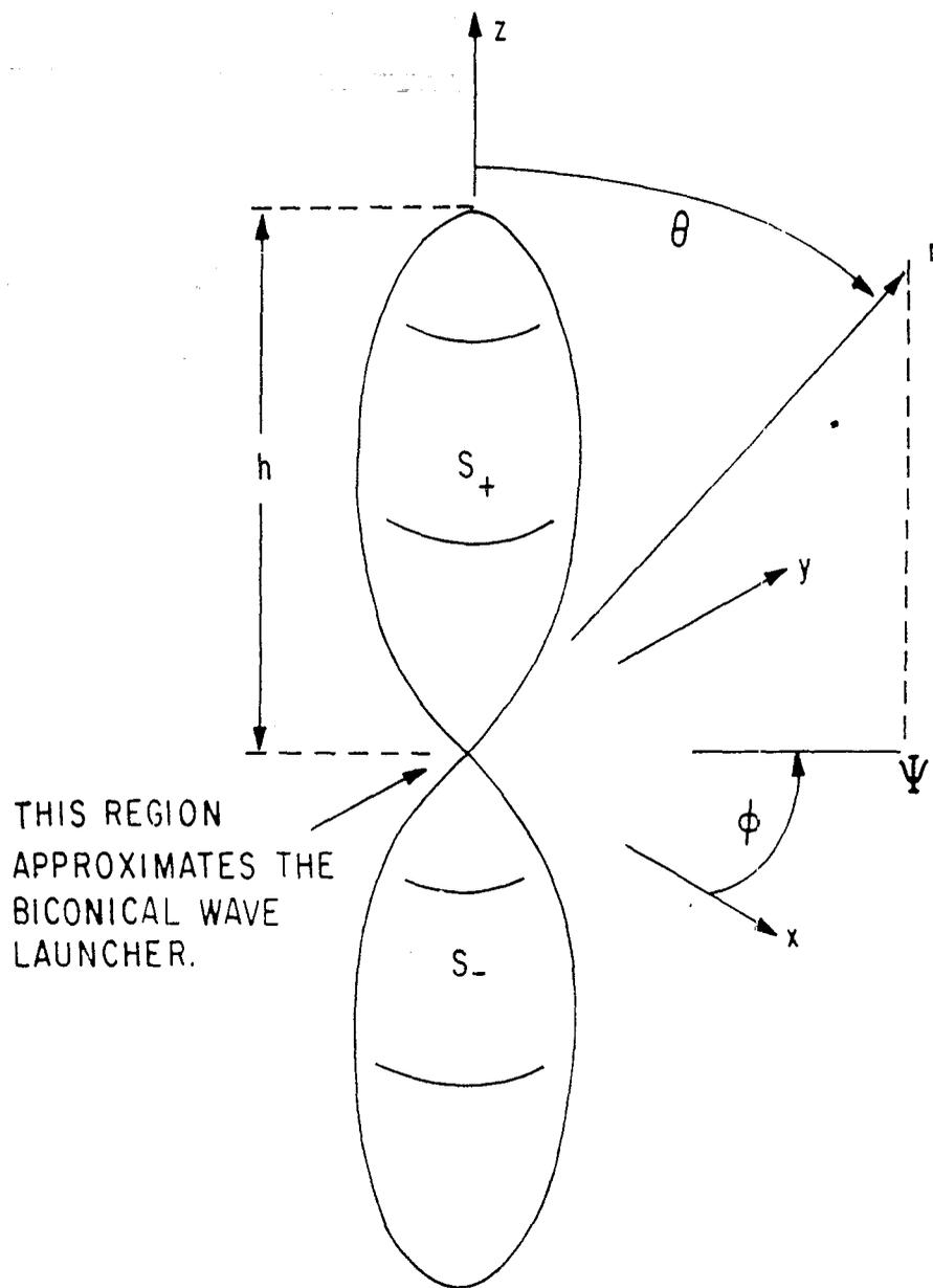
FIGURE I. ANTENNA SURFACES WITH COORDINATE SYSTEMS
