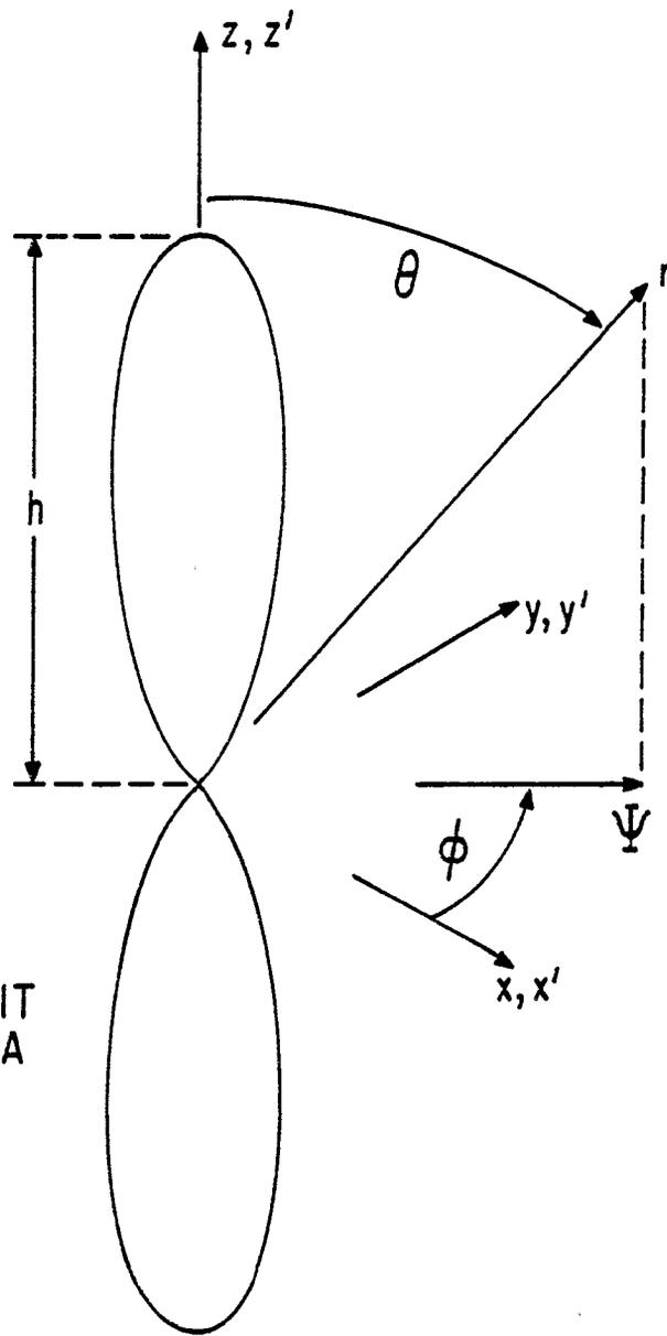
FIGURE 1. AXIALLY AND LENGTHWISE SYMMETRIC DIPOLE ANTENNA
