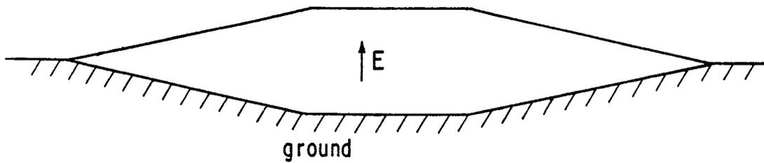
B. VERTICALLY POLARIZED WITH GROUND PLANE SLOPED AT ENDS
