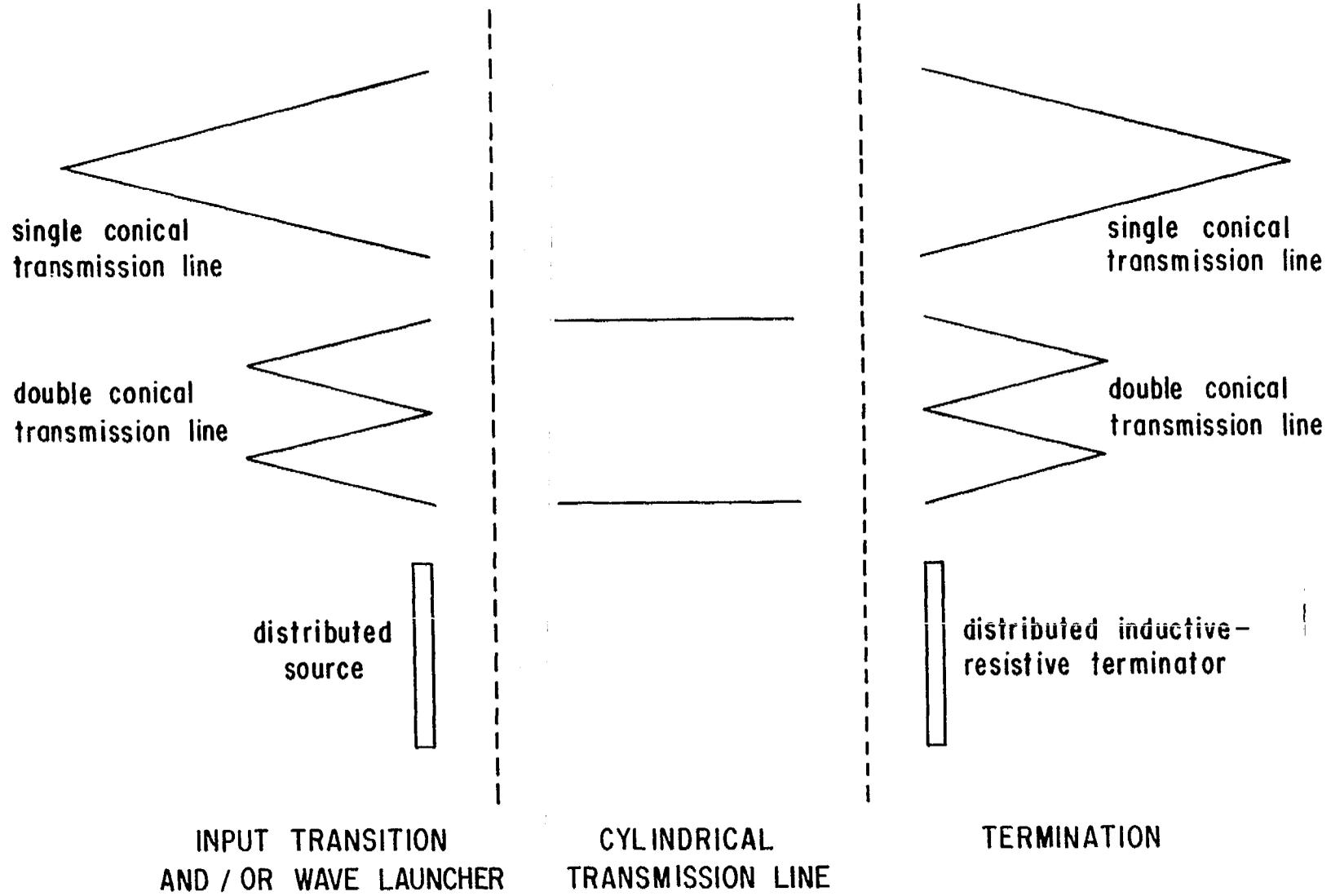
FIGURE 2. SOME OPTIONAL GEOMETRIES FOR PARTS OF A HORIZONTALLY POLARIZED TRANSMISSION - LINE SIMULATOR : TOP VIEW
