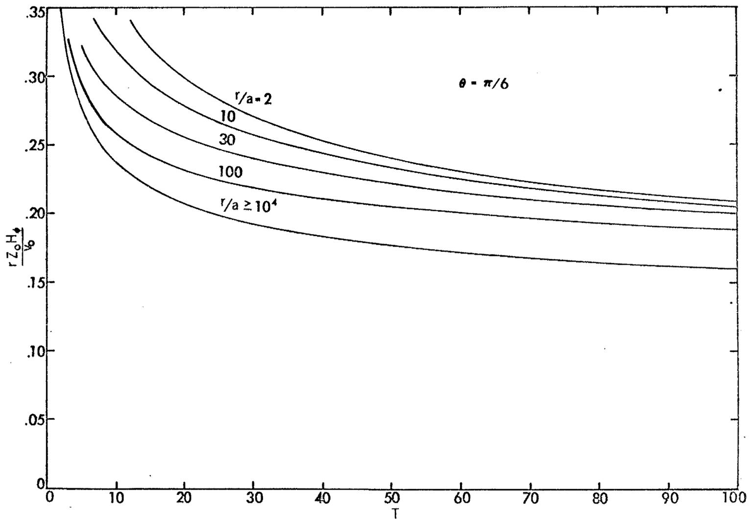
Figure 13. Magnetic-field waveforms for a step-function excitation.
