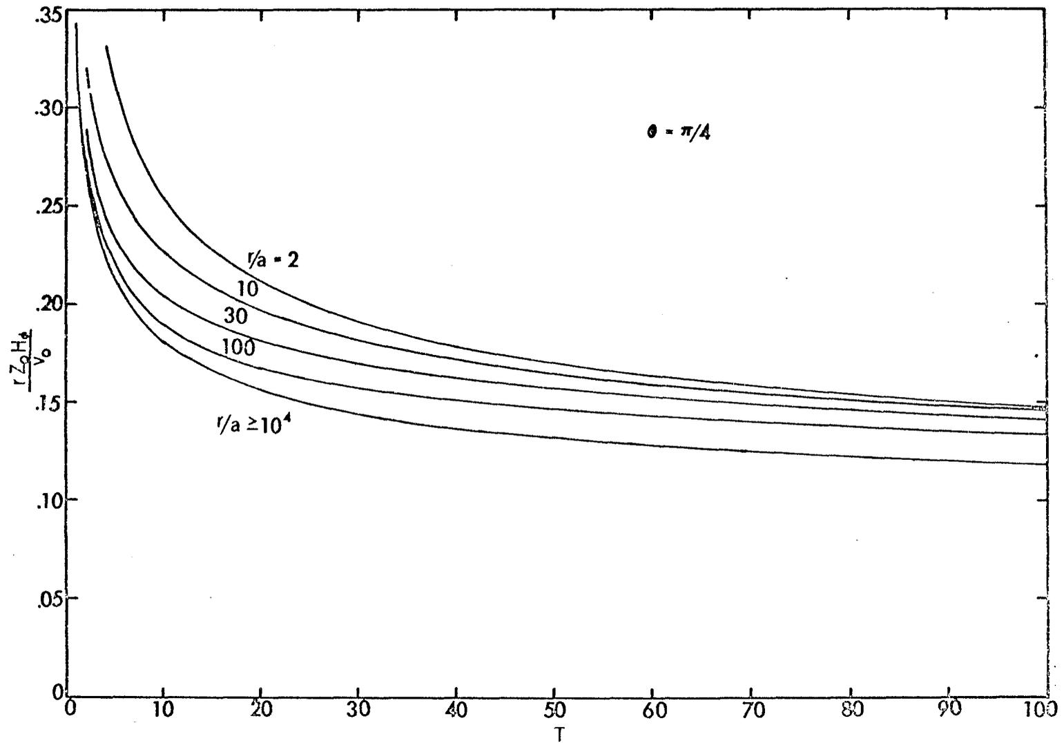
Figure 12. Magnetic-field waveforms for a step-function excitation.
