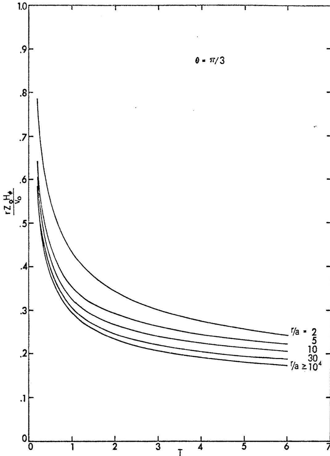
Figure 7. Magnetic-field waveforms for a step-function excitation.
