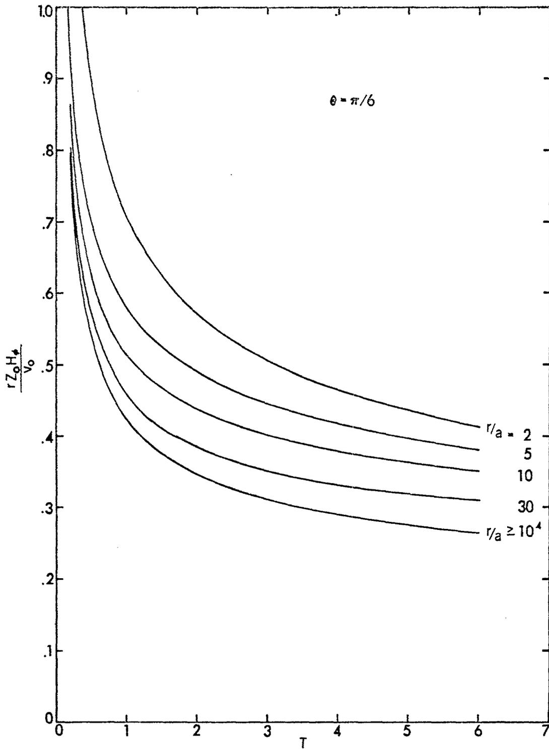
Figure 9. Magnetic-field waveforms for a step-function excitation.
