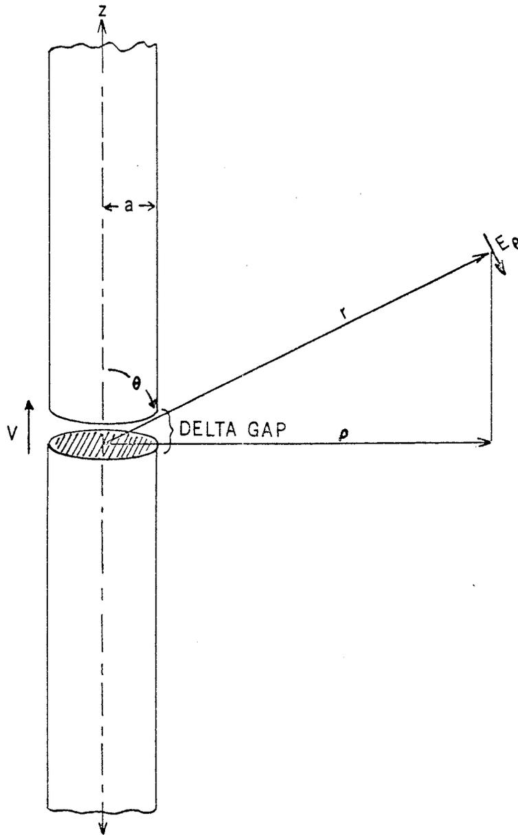
Figure 1. Infinite cylindrical antenna with a gap generator.
