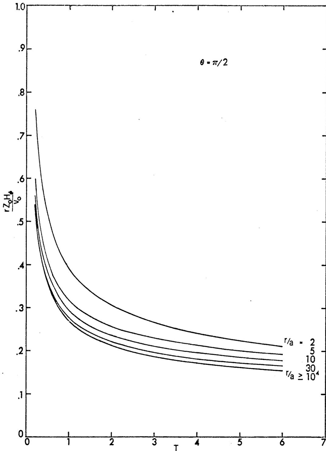
Figure 6. Magnetic-field waveforms for a step-function excitation.
