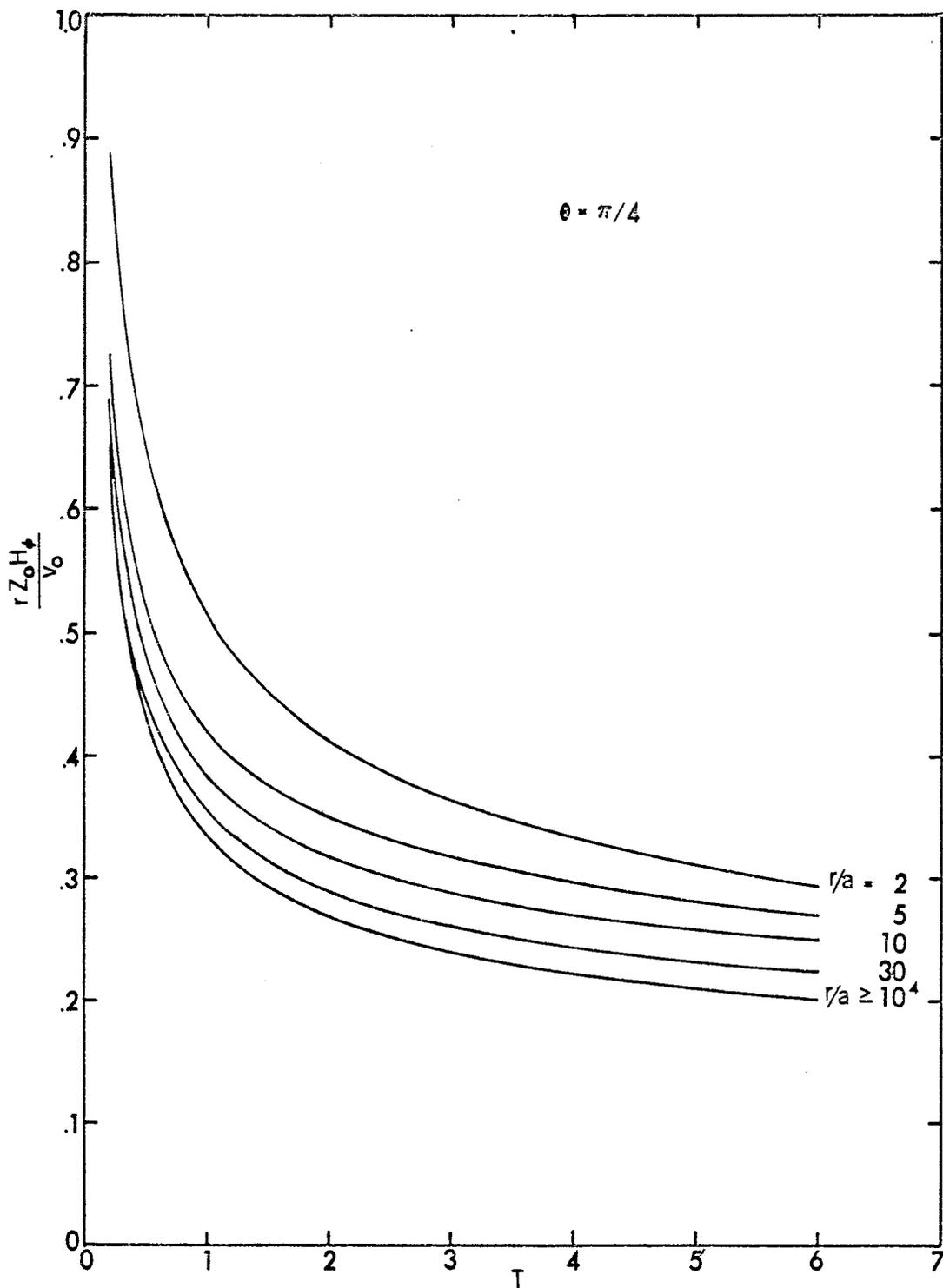
Figure 8. Magnetic-field waveforms for a step-function excitation.
