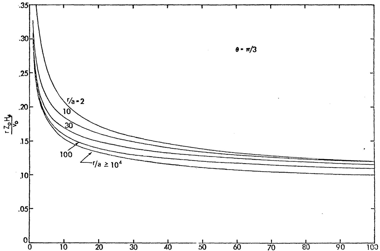
Figure 11. Magnetic-field waveforms for a step-function excitation.
