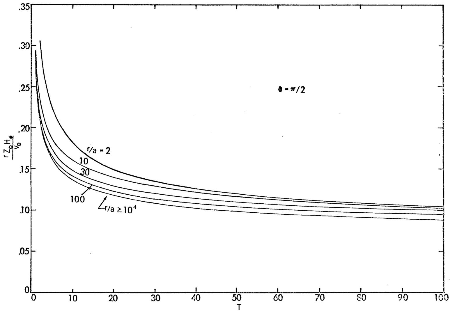
Figure 10. Magnetic-field waveforms for a step-function excitation.
