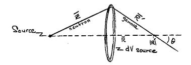
All points in dV emit gammas which reach R at the same time. dV is a ring about the dashed axis. The ionization rate at R and any time, t, is, from Note XI:
