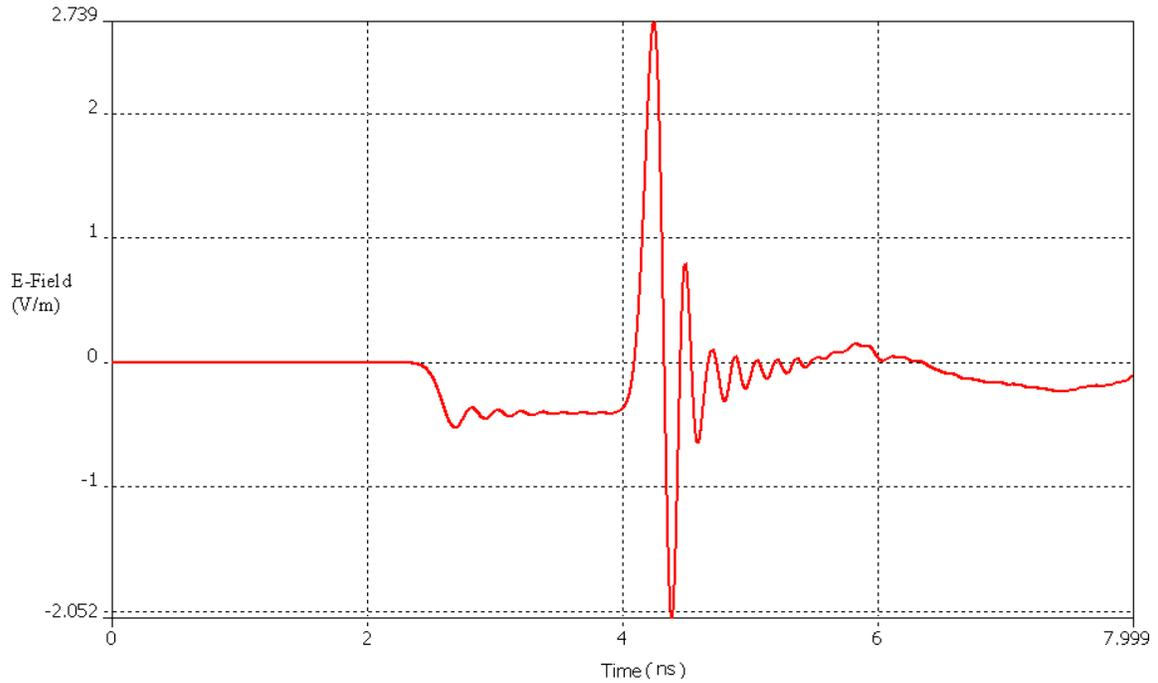
Figure 4.2 Numerical Waveform at the Second Focus at 3GHz & LPW=8
