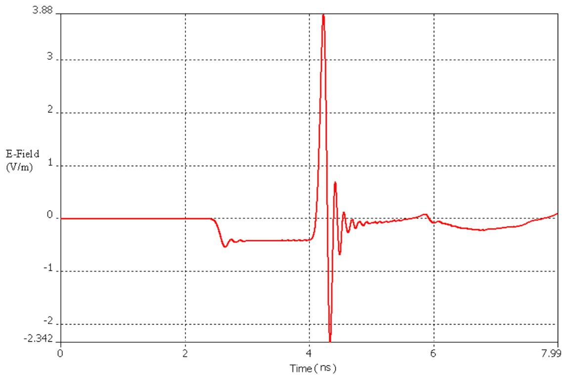
Figure 5.1 Waveform for  $200\Omega$  Resistive Termination
