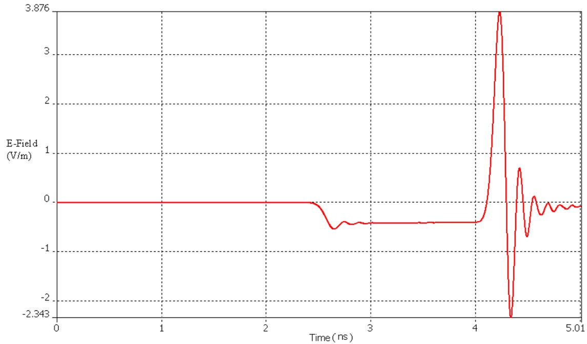
Figure 5.2 Waveform for  $200\Omega$  resistive and  $1\text{pF}$  Parallel RC Termination
