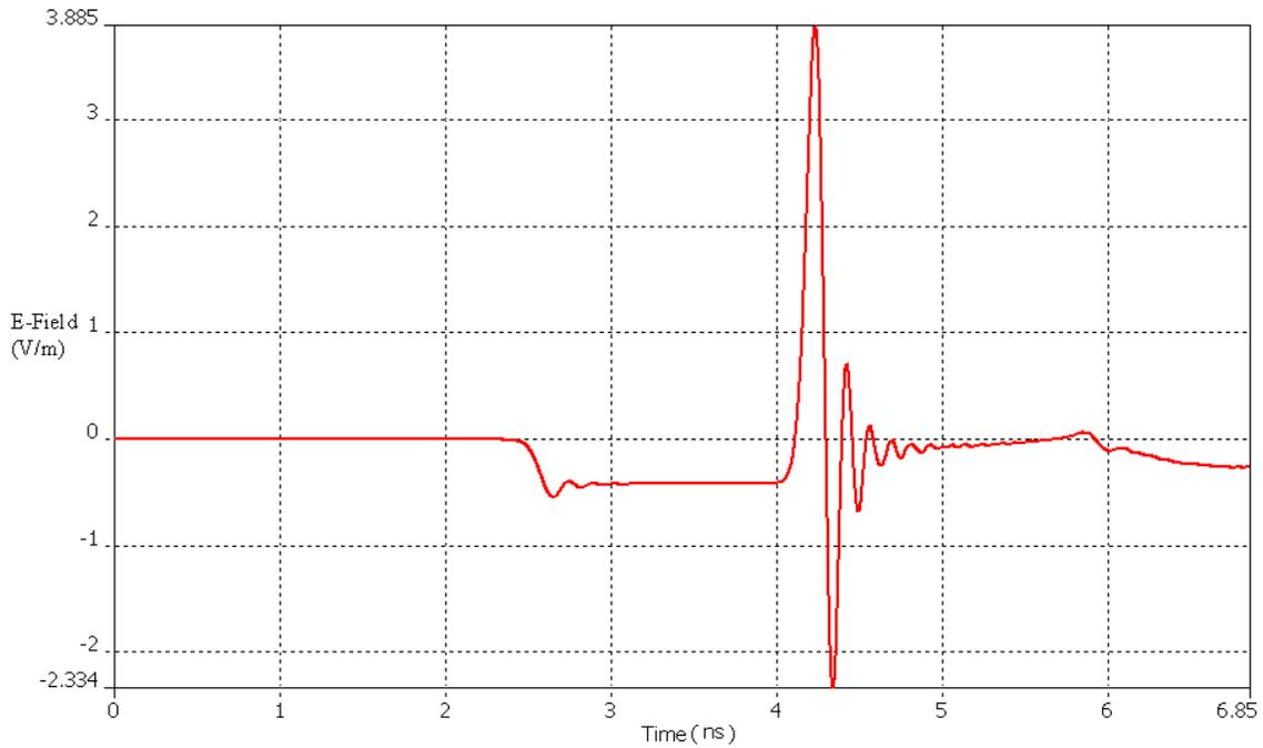
Figure 4.4 Numerical Waveform at the Second Focus at 5GHz & LPW=8
