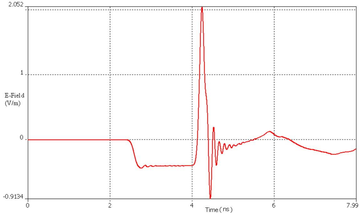
Figure 4.6 Waveform for 200ps at 5 GHz
