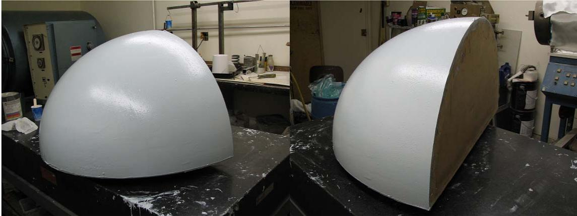
Figure 1: Reflector of the Prolate-Spheroidal IRA
