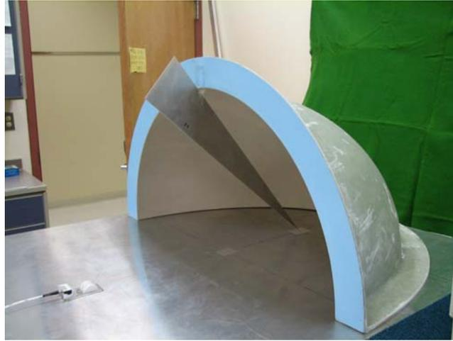
Figure 3: Reflector of a Prolate-Spheroidal IRA
