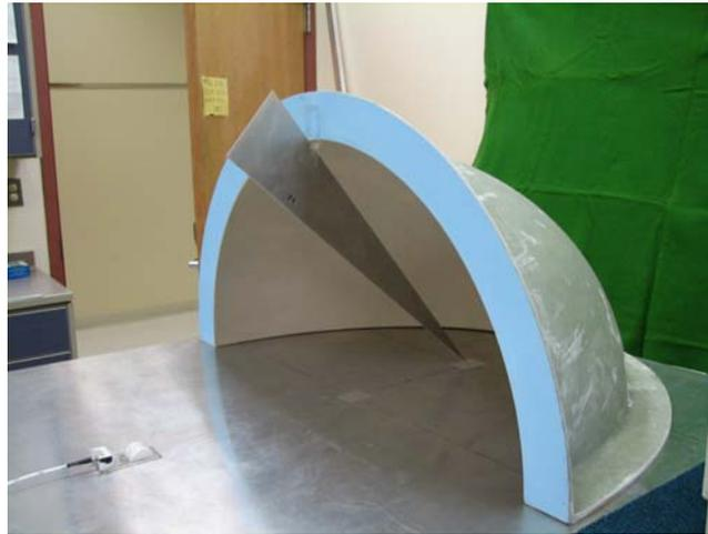
Figure 3: Reflector of a Prolate-Spheroidal IRA
