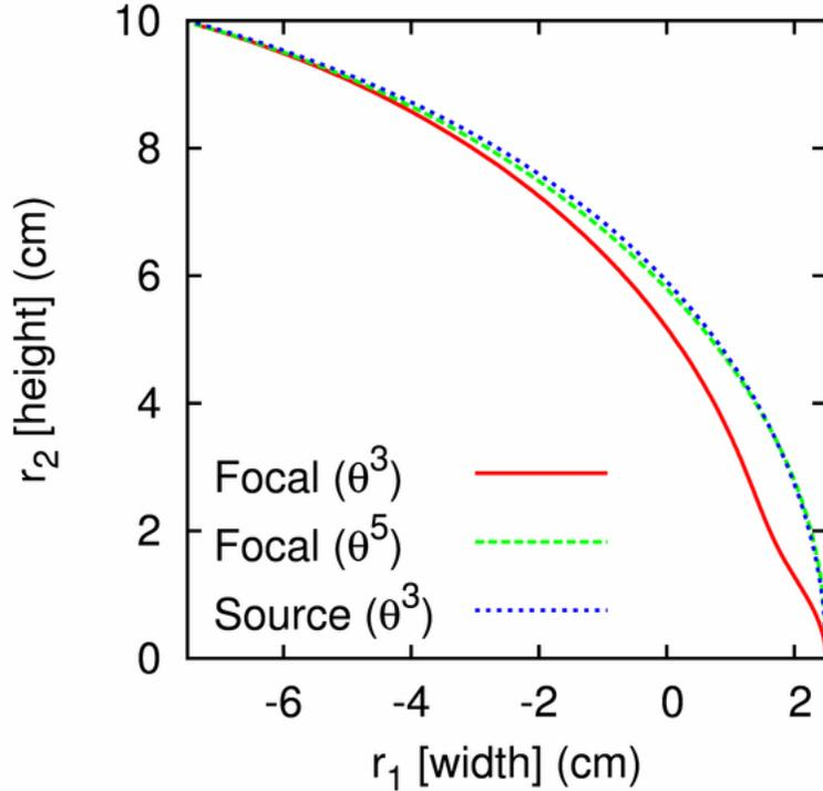
Figure 5.2: Lens boundary curves obtained by using source and focal points as reference. Focal( $\theta^3$ ) is the function  $r(\theta) = a_0 + a_1\theta + a_2\theta^2 + a_3\theta^3$ , Focal ( $\theta^5$ ) is the function  $r(\theta) = a_0 + a_1\theta + a_2\theta^2 + a_3\theta^5$  while Source ( $\theta^3$ ) is  $r'(\theta') = a_0 + a_1\theta' + a_2\theta'^2 + a_3\theta'^3$  using the source as the reference point.
