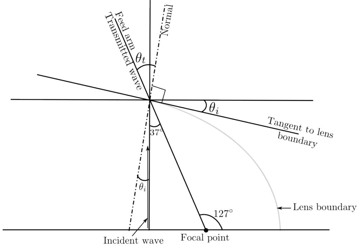
Figure 4.1: Diagram for determination of slope of lens at feed arm angle ( $127^\circ$ )
