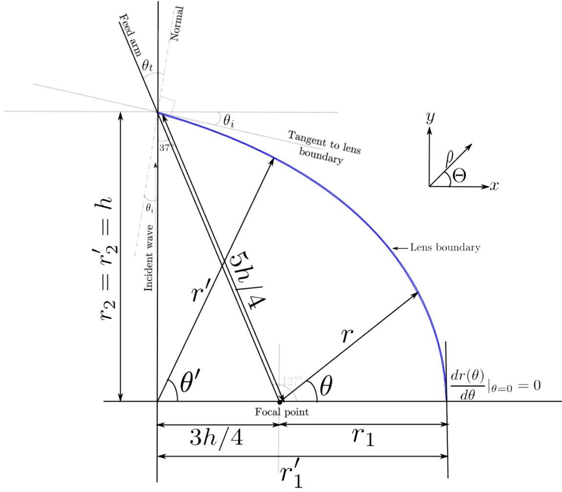
Figure 3.1: Diagram for determination of curve defining lens boundary.  $r, \theta$  refers to the focal point as reference/origin while  $r', \theta'$  uses the source/switch as the reference/origin.
