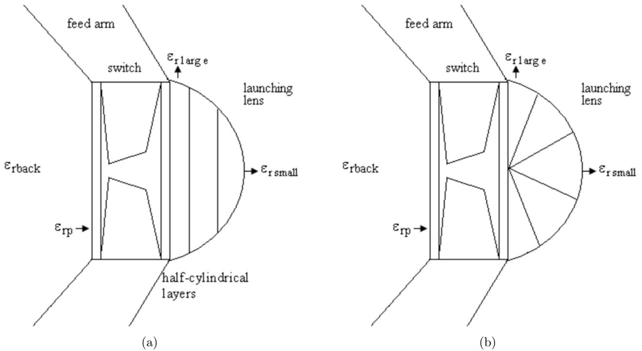
Figure 1.1: Possible configurations of non-uniform launching lens designs
