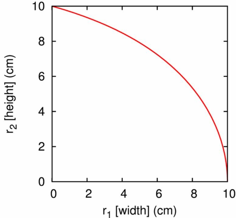
Figure 5.1: Lens boundary curve for function  $r'(\theta') = a_0 + a_1\theta' + a_2\theta'^2 + a_3\theta'^3$  and/or  $r'(\theta') = a_0 + a_1 \sin \theta'^2 + a_2(1 - \cos \theta')$
