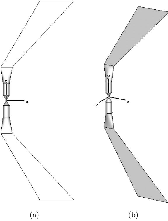
Figure 3.1: Front and perspective views of feed arm and switch with source point at origin
