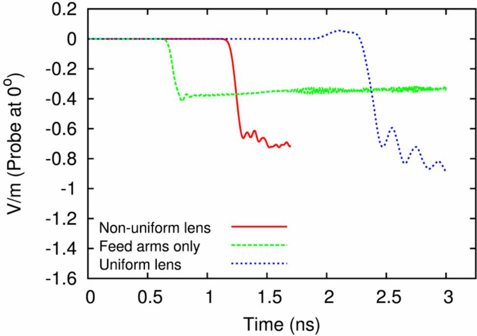
Figure 4.1: Comparison of results for uniform dielectric lens case with non-uniform and feed-arms only cases
