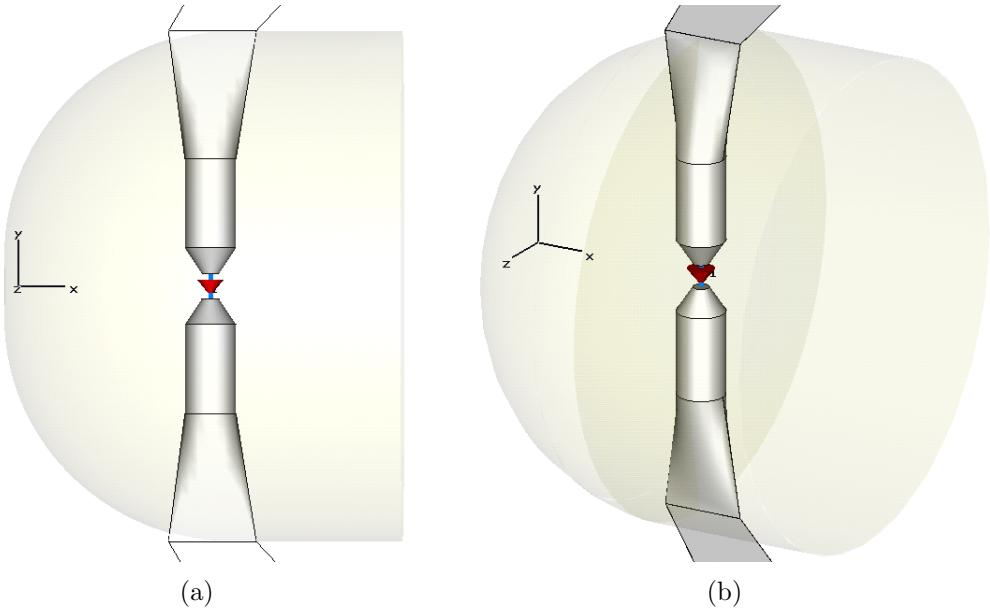
Figure 2.1: Front and perspective views of uniform lens design
