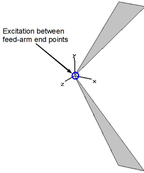
Figure 4.2: Simulation setup with feed arms only and excited at the origin, excitation gap at origin is 4 mm
