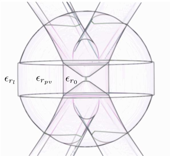
(a) Dielectric constants of switch and pressure vessel system with surrounding dielectric sphere
