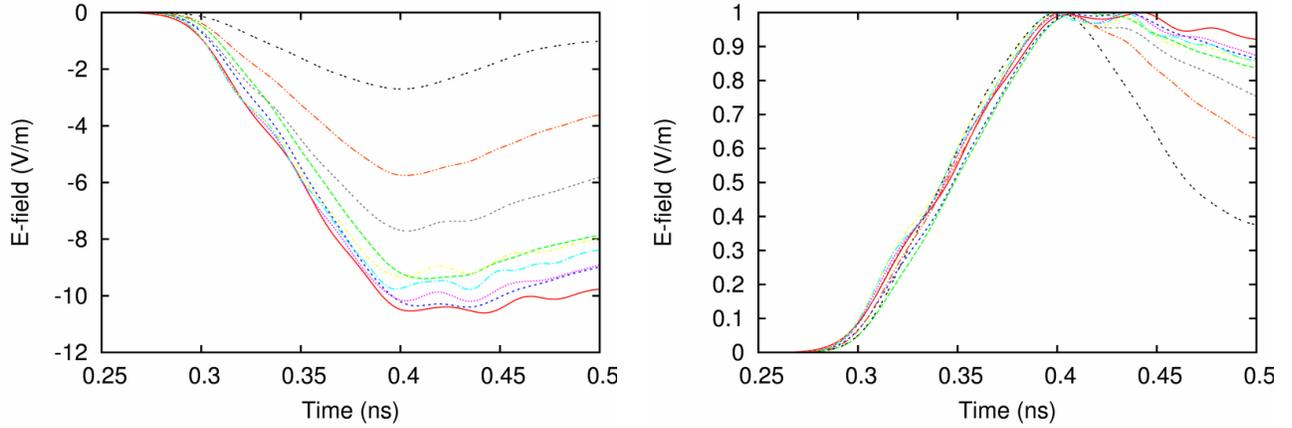
(a) Simulation results for probe orientations in the three planes  $xy, yz$  and  $xz$ . (b) Results normalized with respect to the minimum of each of the wave in (a).
