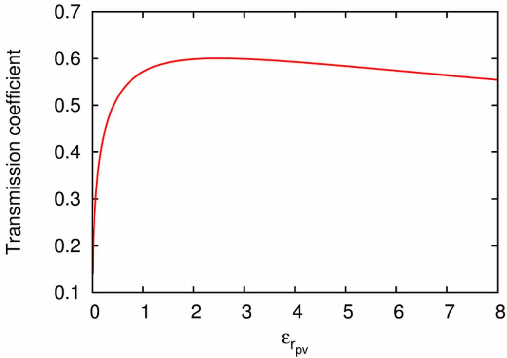
Figure 3.4: Plot of transmission coefficient vs. dielectric constant of pressure vessel.
