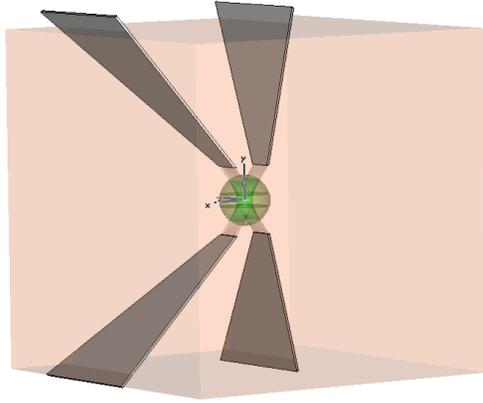
(a) Simulation setup with switch and feed arms immersed in lens dielectric
