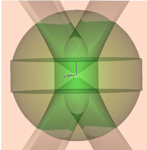
(c) Switch cones, hydrogen chamber, pressure vessel and feed arm connections
