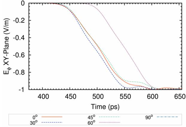
(a) Normalized  $E_\phi$  in the  $xy$ -plane
