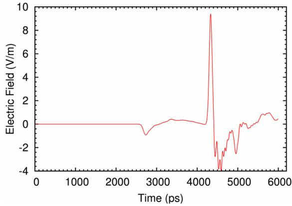
(c) VBCS-IM-75-SPVSHC: Focal impulse waveform.
