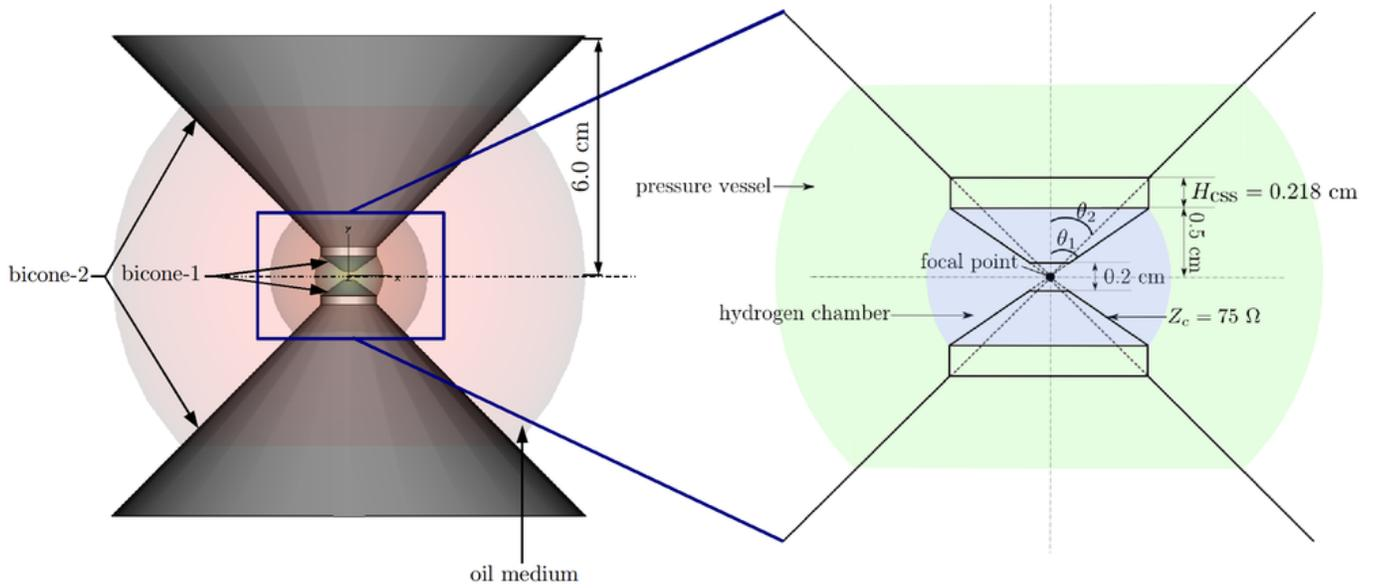
Figure 2.4: Geometrical details and “zoomed-in” side view of switch system for the VBCS-IM-75-SPVSHC configuration.
