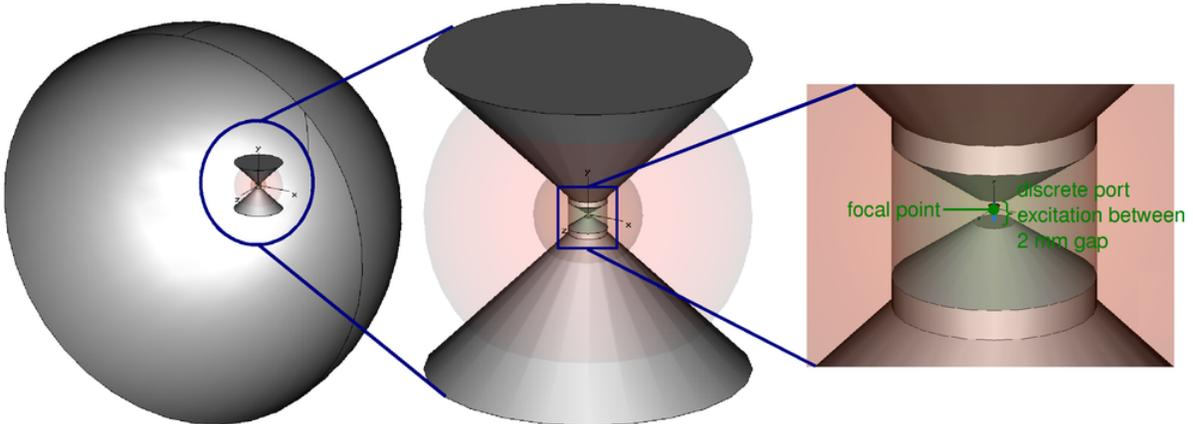
Figure 2.1: Perspective view of VBCS-IM-75-SPVCHC configuration with reflector; “Zoomed-in” view showing discrete port excitation.
