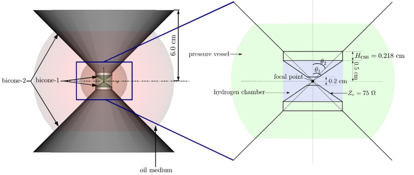
Figure 2.2: Geometrical details and “zoomed-in” side view of switch system for the VBCS-IM-75-SPVCHC configuration.
