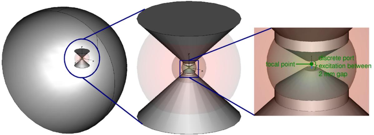
Figure 2.3: Perspective view of VBCS-IM-75-SPVSHC configuration with reflector; “Zoomed-in” view showing discrete port excitation.
