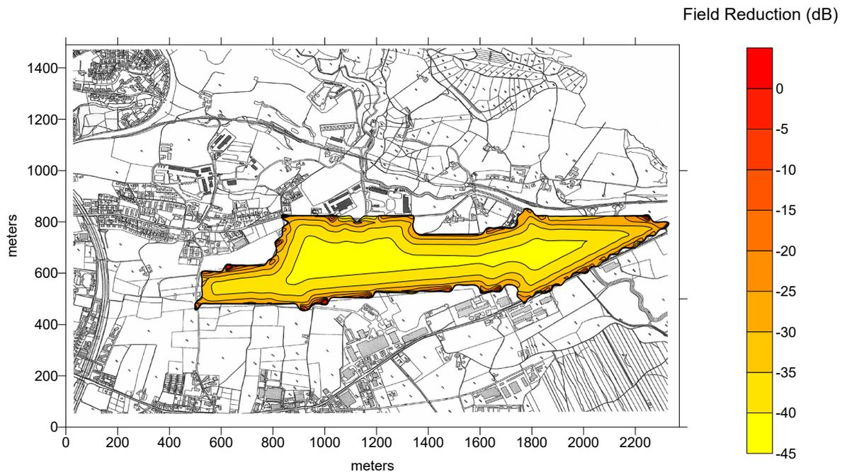
**Figure 14. Contour plot of the E-field reduction factor (in dB) for points inside the access-controlled region of the airport, for radiating antennas located at the boundary.**
