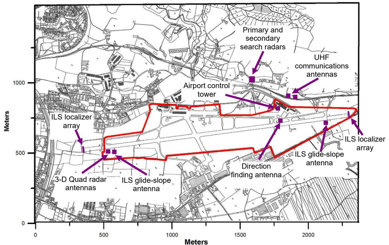
**Figure 13. Map of the airport and surroundings, with the access control perimeter and major antennas indicated.**
