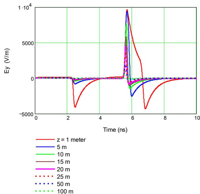
**Figure 11. Plots of the principal component of the transient SWIRA E-field at different observation ranges ( $z$ ) from the antenna.**
