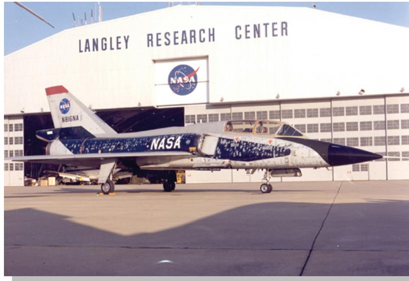
**Figure 2. F-106B (NASA 816) research aircraft during Storm Hazards Program in 1982. (Note paint spots applied to aircraft that denote lightning attachment points.)**
