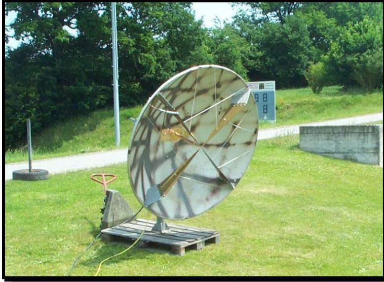
**Figure 10. Illustration of the Swiss Impulse Radiating Antenna (SWIRA).**
