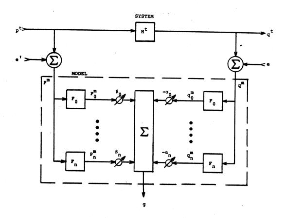
Figure 2.2. Generalized model of a linear system. e' and e are measurement error sequences.
