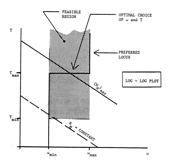
Figure 4.1. Guidelines for choosing sampling rate and period of observation for resonance extraction.
