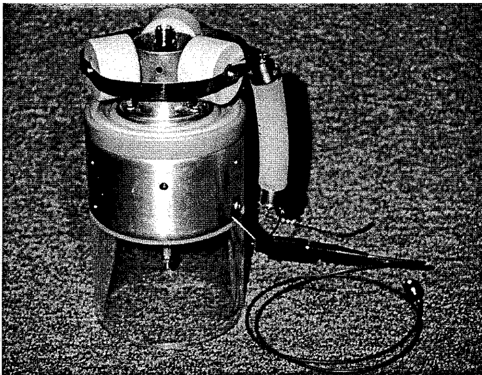
Figure 4.3. Assembled High-Voltage, High-Pressure Switch
