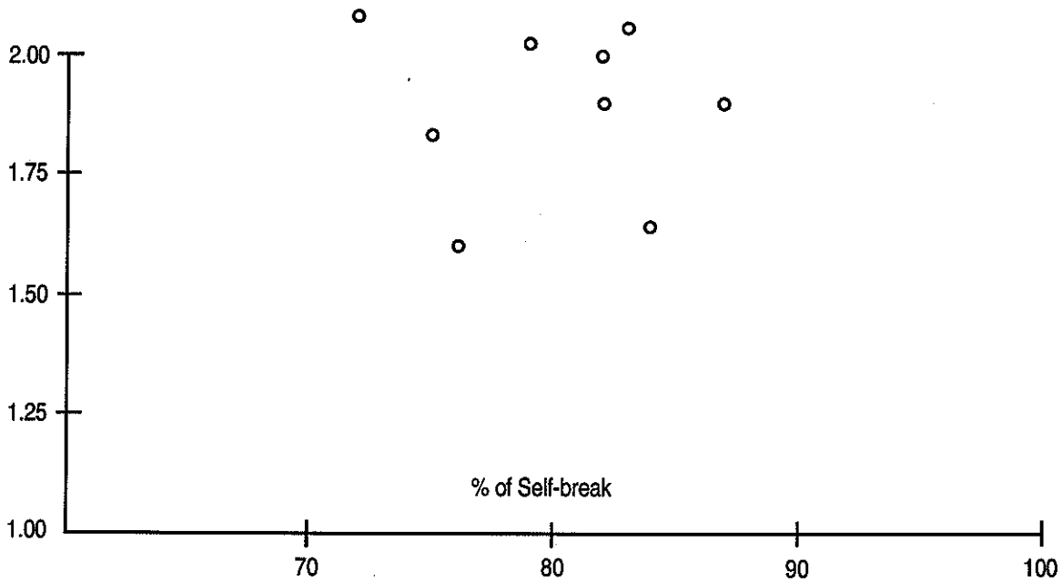
Figure 93. TS closure delay as a function of % of self-break; TS gap 0.257 cm, nitrogen gas, mushroom stick-out 33% (data from Table 10).
